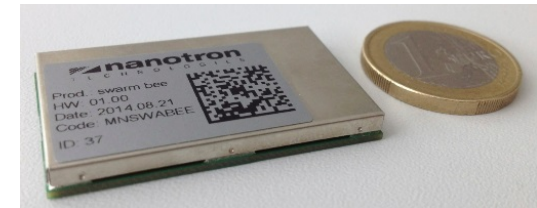
swarm bee module 24 x 40 x 3,5 mm 3 available with CSS and UWB
