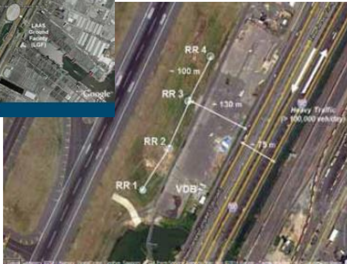
FIGURE 8 LAAS Ground Facility site at Newark Airport showing GBAS antenna locations
