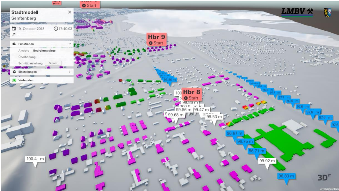
Figure 5 Digital terrain and city model plus integration of large-scale technical systems and sensors; query via OPC/UA interface in 3D real time; control possible; extrapolation of third variables (sectional views possible, also display of documents (digital twin). Courtesy of the project partners LMBV and UBV
