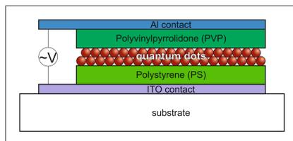
Fig. 1: Schematic of a QLED
