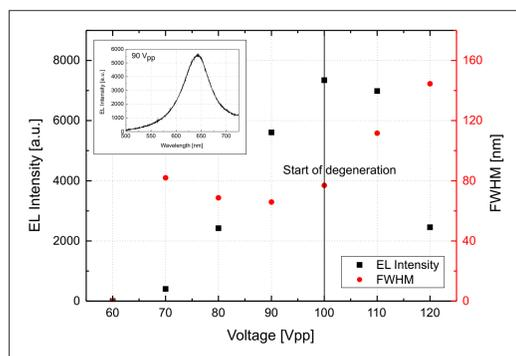
Fig. 3: Electroluminescence (EL) intensity and FWHM of a QLED at different applied voltages
