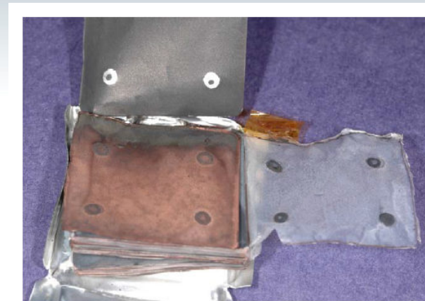
The anode of a repeatedly over-discharged cell coated with copper.
