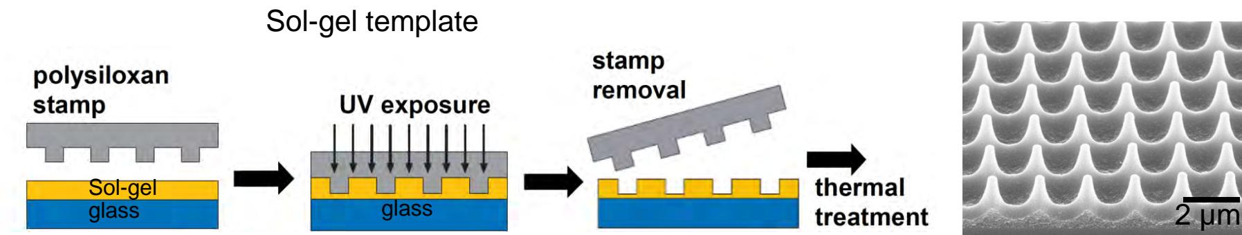
Simple large area fabrication with precisely controlled nanoscale dimensions
