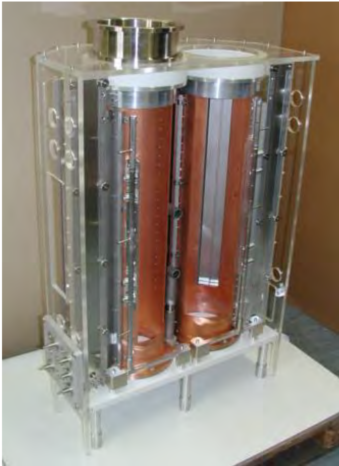
a) Serial co-sputtering source (model)
