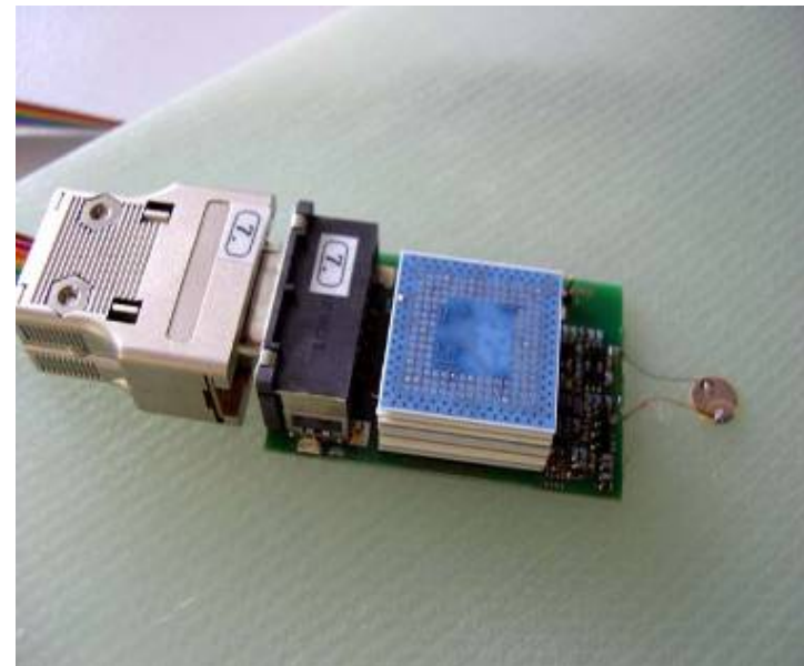
Impact detection system based on Match-X standard CAN-Bus network
