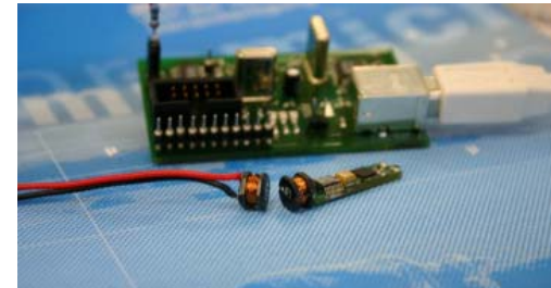
Inductive generators (Fa. pro-micron)
