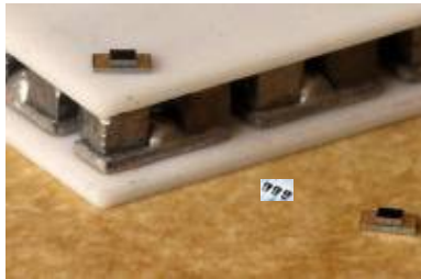
Thermo-generators (Fa. Micropelt / FhG IPM)
