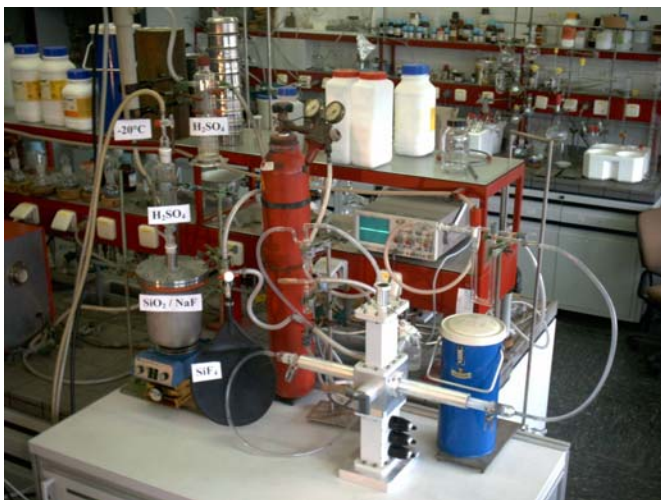
Laboratory scale device for microwave assisted polysilane and silicon production
