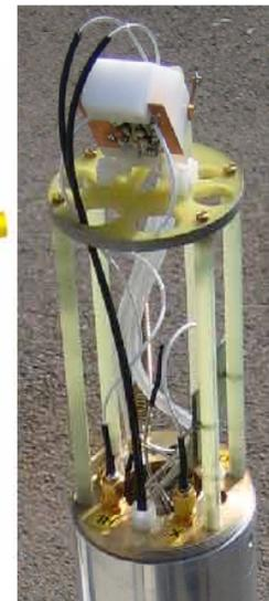
Positioning of detection coil at the "magnetic center" (maximal field strength and highest field homogeneity)
