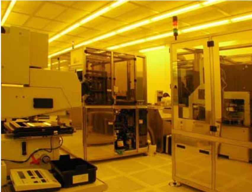
Cluster for resist deposition (spin on and spray coating), exposure, develop and bake
