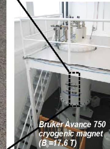
Bruker Avance 750 cryogenic magnet ( $B_0=17.6\text{ T}$ )
