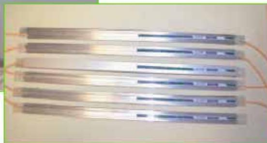
FBG sensor pads with strain
