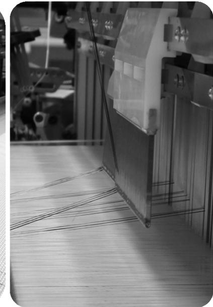
Detail B: needle bar with CFY in open shed position
