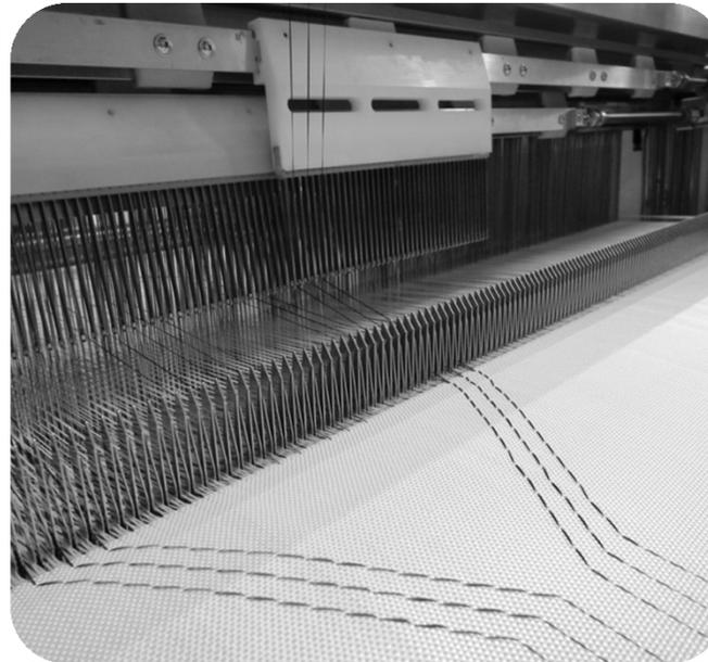
Detail A: linear drive unit with needle bar and Open Reed Weave (ORW<sup>®</sup>)
