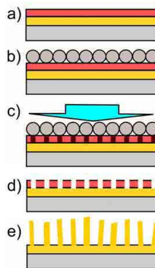
...by nanosphere photolithography – finite-difference time-domain (FDTD) simulation  $\lambda = 405 \text{ nm}$
