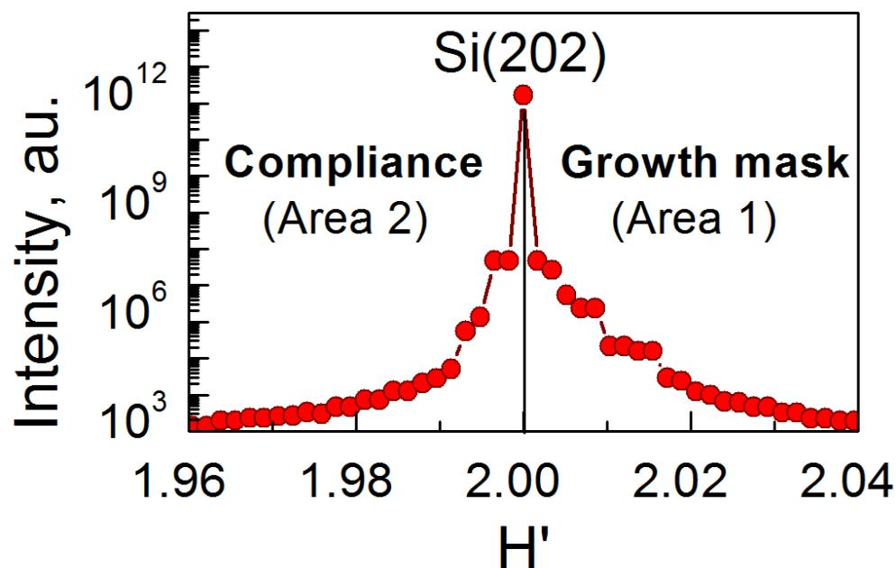
(202) Bragg reflection – Strain in Si nanopillar
