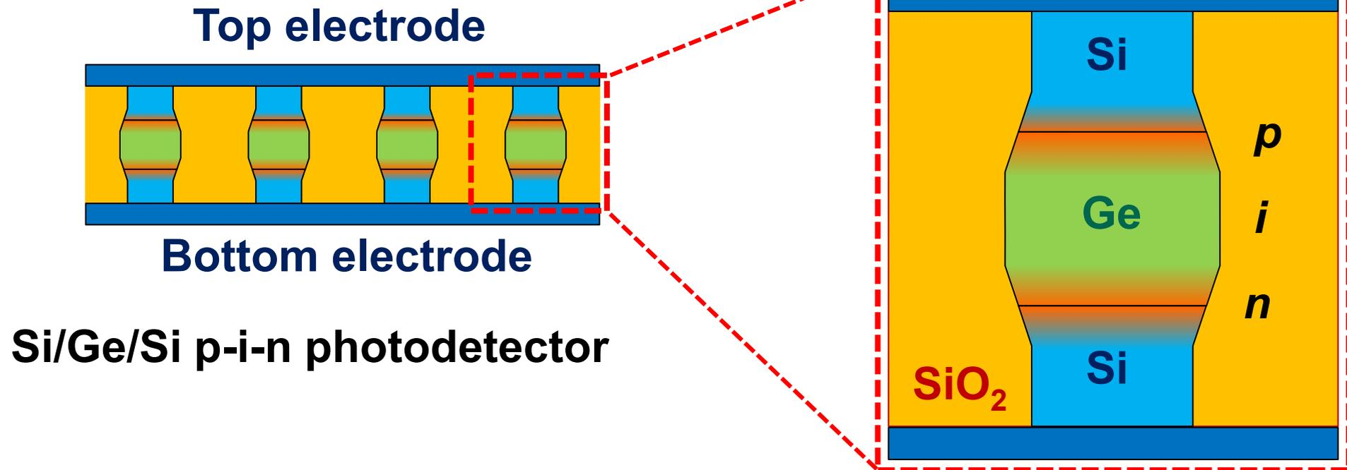
**High-speed and high-power photodetector is a must**
