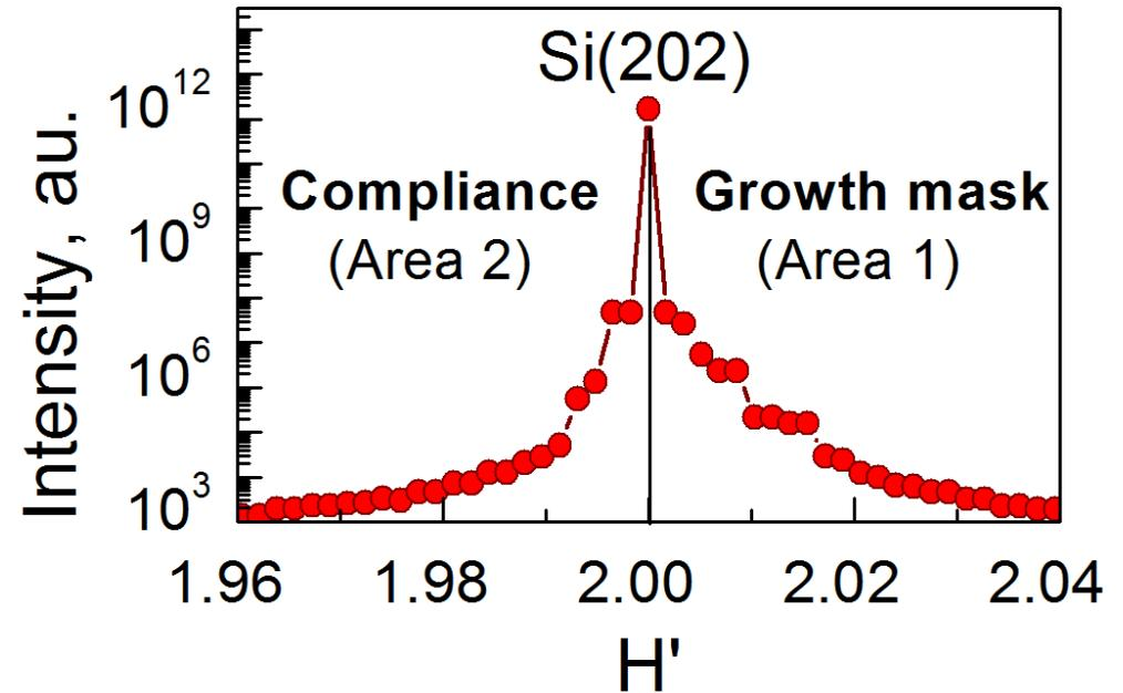
**(202) Bragg reflection – Strain in Si nanopillar**
