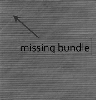
missing bundle |
