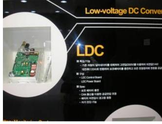
DC-DC Power Converter 300V -> 14V, 120A
