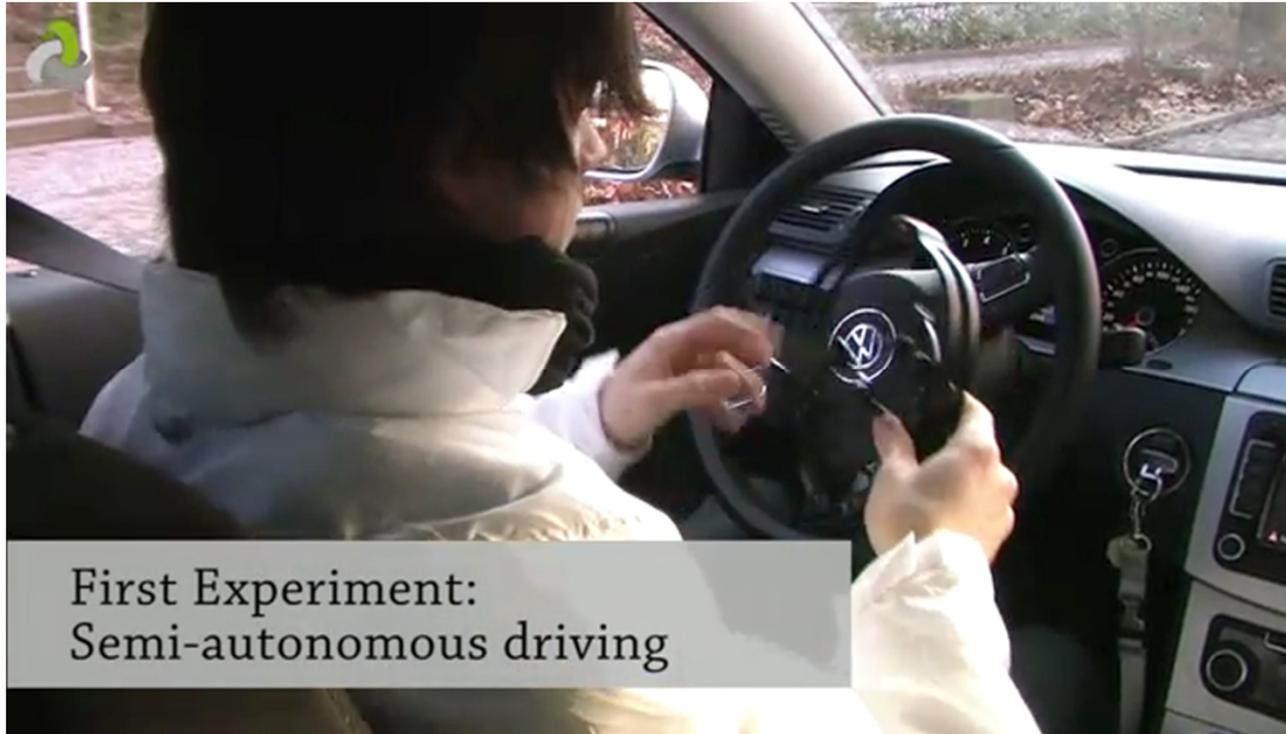
After testing an iPhone, an iPad and an eye-tracking device as possible user interfaces to maneuver our research car named [“MadeInGermany”](#), we now also use brain-power. Neuro-signals are acquired using the commercial Emotiv EEG (electroenzephalogram) tool.
