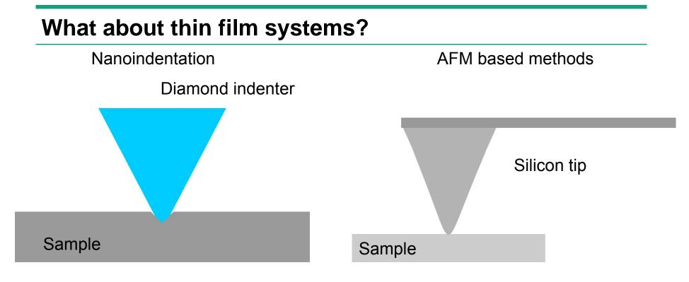
Force range: 100 nN – several mN Tip radius: 100 nm – 500 nm -  $20 \mu \text{m}$ Film thickness limit : ca. 200 nmIndentation depth: 5 nm –  $20 \mu \text{m}$  Force range: 1 nN – several  $\mu$ N Tip radius: 10 nm – 150 nm – 500 nmFilm thickness limit : ca. 50 nm
