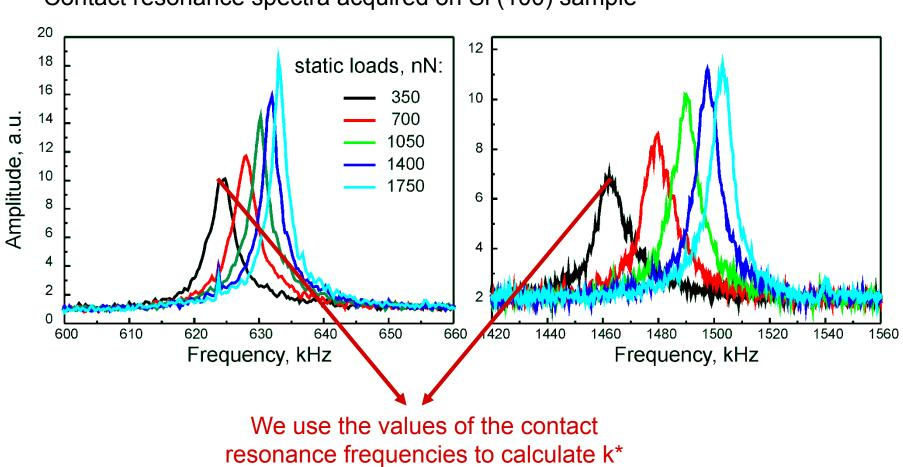
Contact resonance spectra acquired on Si (100) sample
