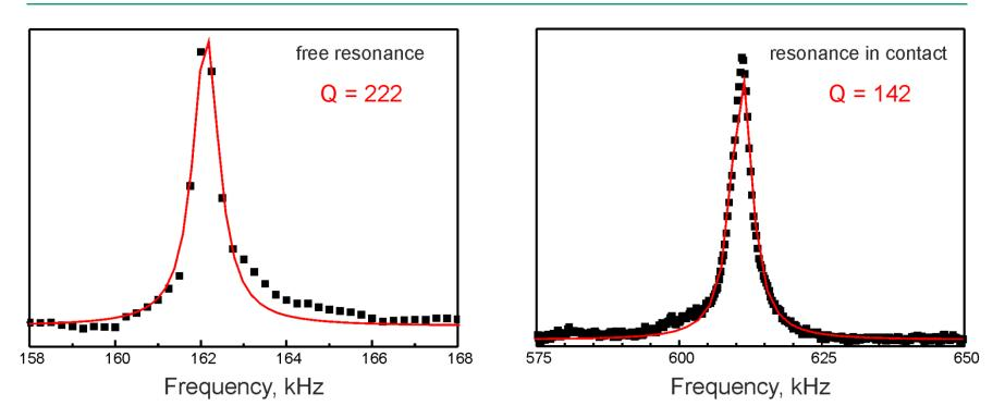
From the analysis of the resonance spectrum we can determine values of the contact resonance frequencies, Q factor, and damping of the cantilever in air
