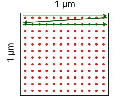
The values of contact resonance frequencies are determined as a function of a position on the sample surface at a fixed value of the applied static load.
