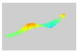
Cantilever vibrations measured at IZFP-Saarbrücken
