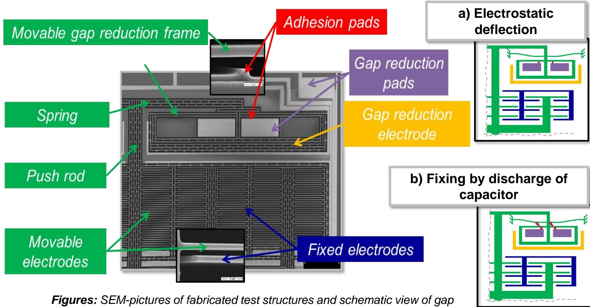
**Figures:** SEM-pictures of fabricated test structures and schematic view of gap reduction procedure
