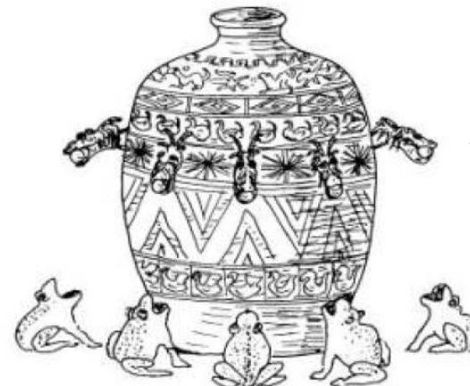
**Figures:** Replica and picture of Zhang Heng's seismoscope
