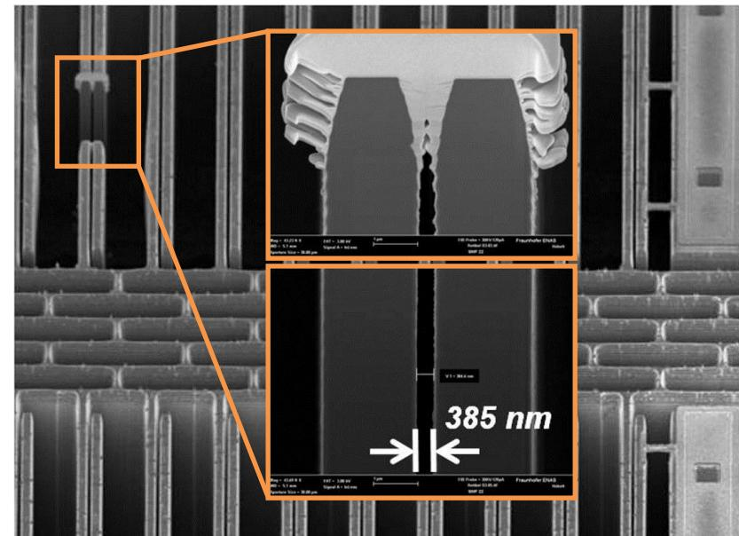
**Figures:** SEM photographs after FIB preparation (overview of comb electrodes and detailed view of an electrode pair)
