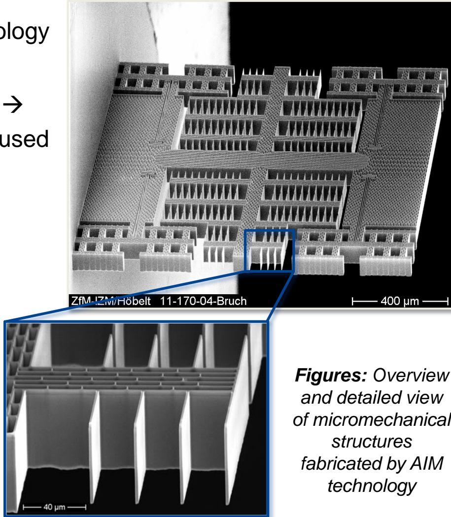
**Figures:** Overview and detailed view of micromechanical structures fabricated by AIM technology
