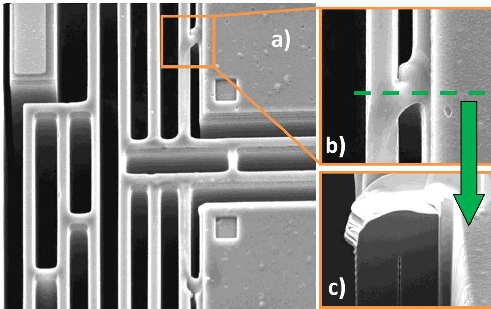
**Figures:** SEM photograph of a gap reduction area after the gap reduction sequence has been done a) including a top view of a micro welding pad b) and a cross section of a micro welding pad after FIB preparation c)
