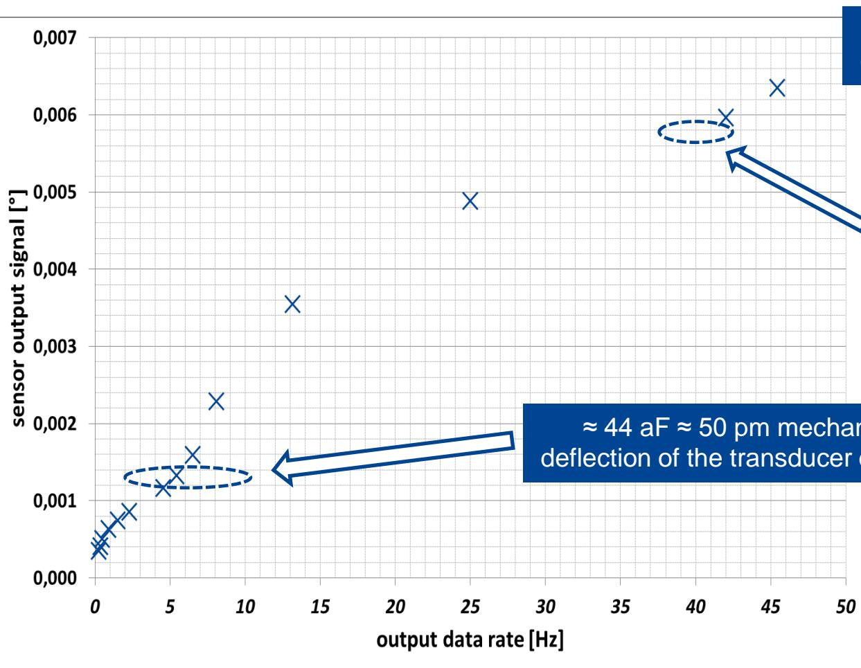
$\approx 165 \text{ aF} \approx 200 \text{ pm}$  mechanical deflection of the transducer element
