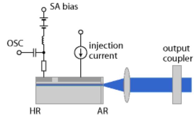
(b) device with modulated absorber section
